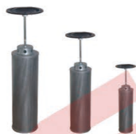
XNL Tank Mounted Return Line Filter Series Flow rate: 25-1000L/min Pressure: 0.6MPa Precision: 1-30µm Dia.: 20-90mm Connecting: Flange Element Model: NLX Series
