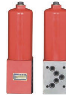
DF Superimposed Filter Series Flow rate: 30-110L/min Pressure: 32 MPa Precision: 3-20µm Dia.: 6mm 10mm Connecting: Thread, Flange Element Model: LH Series
