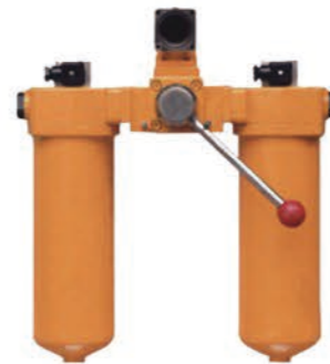
ZU-A SQU-A SWU-A SXU-A Duplex Return Line Filter Series Flow rate: 25-400L/min Pressure: 1.6 MPa Precision: 1-30µm 50µm (only SXU-A) Dia.: 20-65mm Connecting: Flange Element Model: STZX2 Series STXX Series
