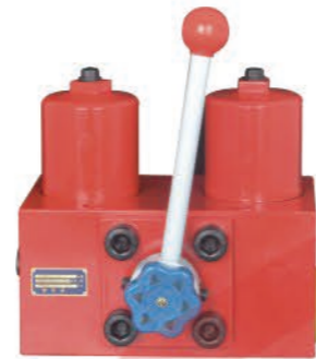
SGF Duplex High Pressure Line Filter Series Flow rate: 30-660L/min Pressure: 32MPa Precision: 3-20µm Dia.: 20-50mm Connecting: Flange Element Model: LH Series
