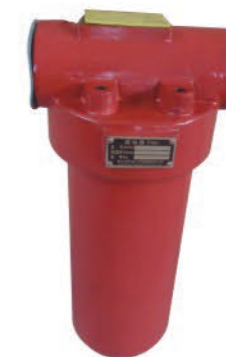
GU-H Tank Mounted Pressure Line Filter Series Flow rate: 10-630L/min Pressure: 32 MPa Precision: 3-40µm Dia.: 15-55mm Connecting: Thread, Flange Element Model: GX Series
